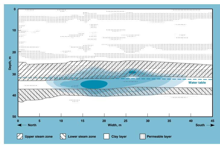
Figure 5. Approximate cross section of the treatment site after the two steam passes (compare with Figure 1). The area of gasoline contamination has contracted greatly.
