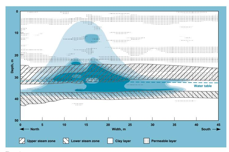
**Figure 1.** Cross section showing an approximation of the gasoline contamination at the treatment site before dynamic underground stripping began. The darker areas represent higher concentrations or free-product gasoline. The dashed line denotes the level of the water table.
