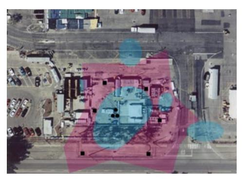
**Figure 2.** Top view of LLNL spill area, showing regions of known or suspected free-product gasoline contamination (circled in blue) and where we applied dynamic underground stripping (in pink). As noted by the circles outside the treatment area, additional free-product gasoline remains at the site.
