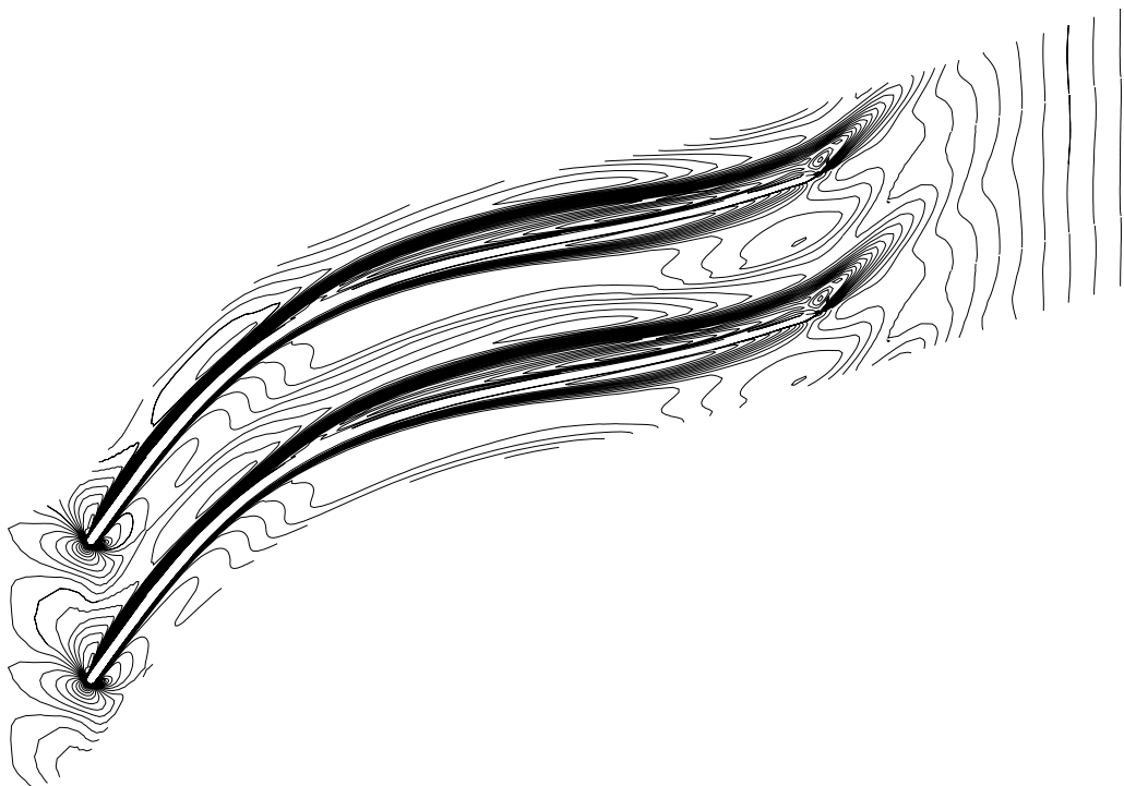
Figure 3 – Mach contours for a centrifugal impeller rotor.
