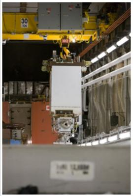
Technicians use a crane to lift NuMI horn 2 out of
