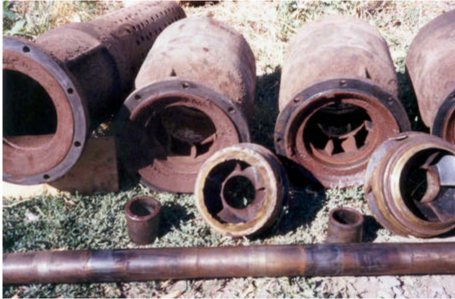
Figure 2. OIT #5 suction case, 1st and 2nd bowls, and 2nd and 3rd impellers.
