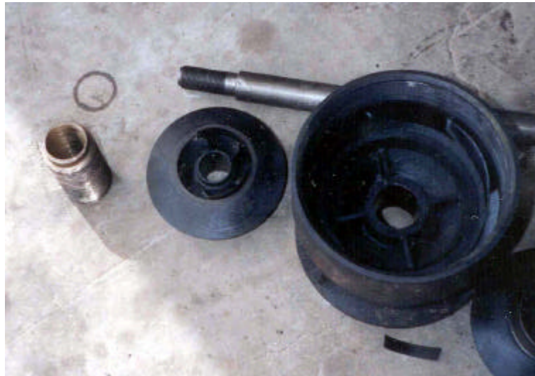
Figure 8. Left to right bottom: oil tube brg., top impeller, top bowl, and 2nd impeller from top.
