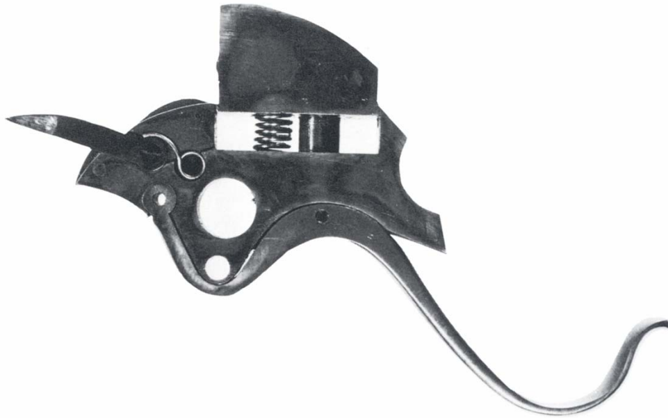
Guard lever and breechblock assembly
