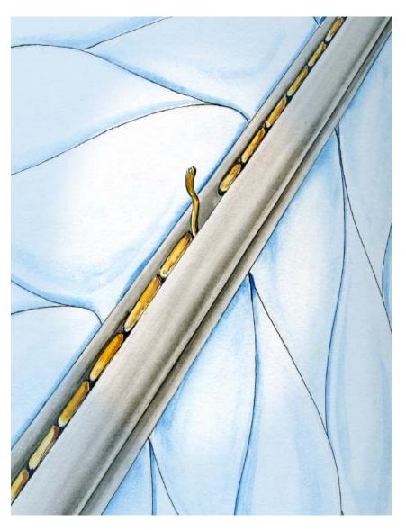
Broken stitches represent a rupture of either the top or bottom thread.
