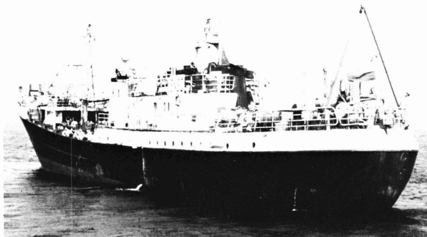
Figure 1.—Polish research vessel Wigry , 61 m long. Jigging gear is on the well deck.
