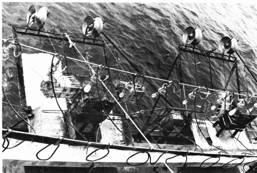
Figure 5. —Overhead view showing 2,000-watt and 4,000-watt lamps suspended over the jigging machines.
