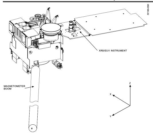
Figure 5-2. Deployed XRS/EUV Instrument—Schematic View
