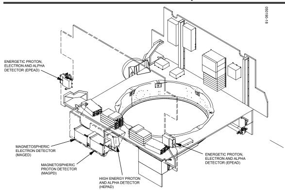
Figure 5-4. EPS/HEPAD Instrument Locations
