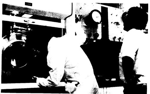
BURN, BABY! BURN!—Mike Mannon and Frank Melendrez monitor an upward propagation burn test in 30 percent oxygen of a swatch of fluorosilicone rubber in one of WSTF materials test lab's small chambers.
