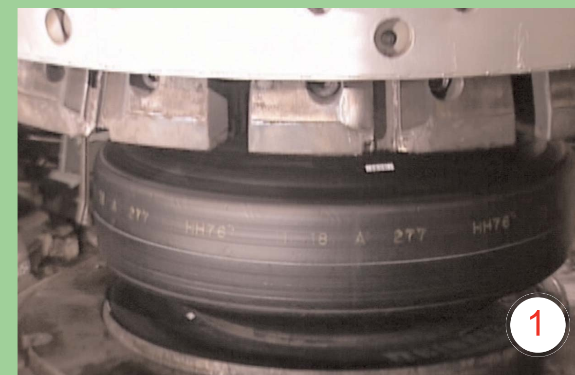
1 Tires are cured by placing an uncured (green) tire into a tire mold.
