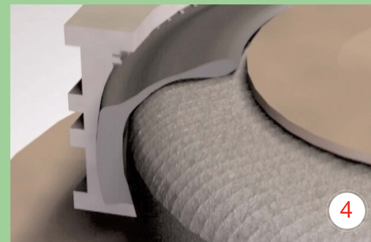
4 The mold is heated with steam in order to provide the heat necessary to cure the tire.
