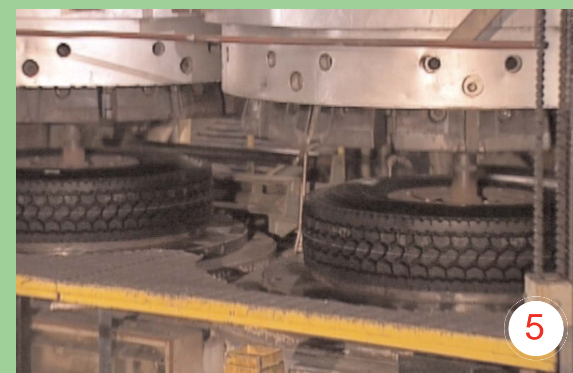
5 When the press opens the cured tire is revealed.
