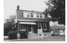
The brick and concrete utility building, 40 feet by 20 feet by 16 feet, constructed in 1939, contains a workroom, garage, implement room and two public toilet rooms. The roof is tile.
