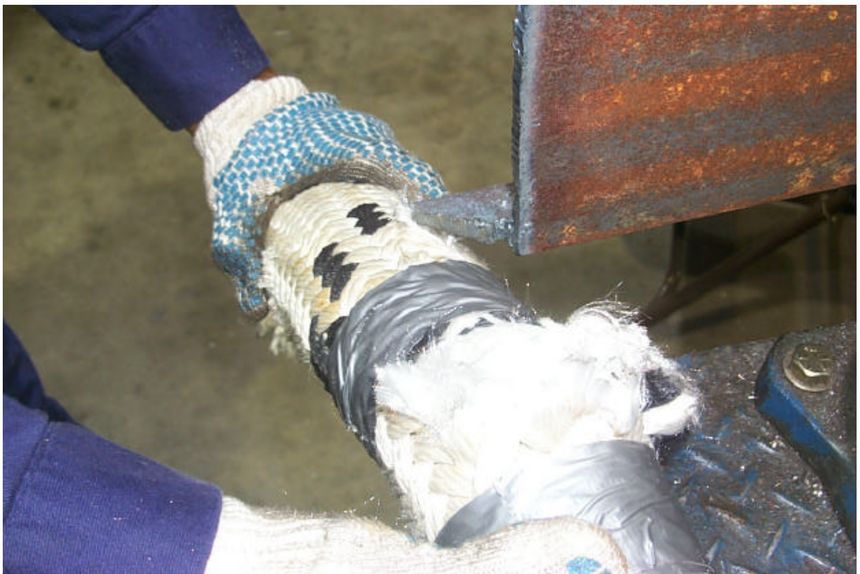
Figure 6. Puncture test with raw edge of steel angle.
