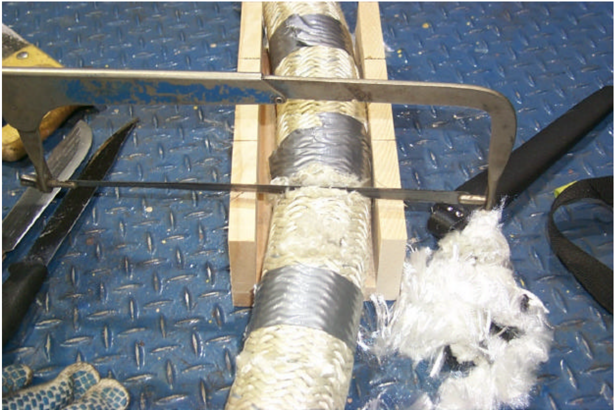
Figure 5. Cutting with hacksaw.
