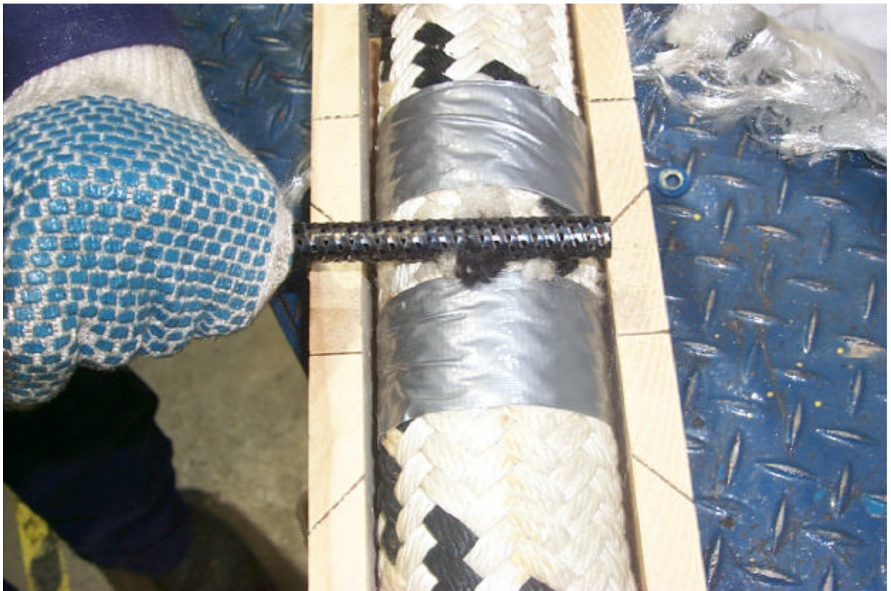
Figure 4. Cutting with piece of reinforcement bar.
