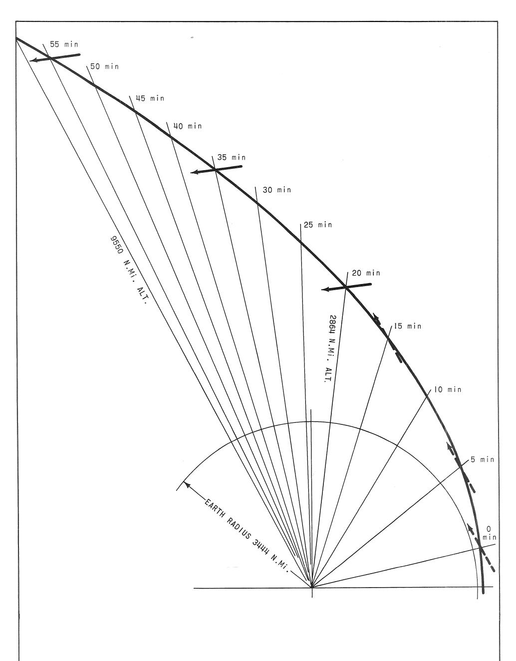
FIGURE | POST INJECTION ALTITUDE PROFILE
