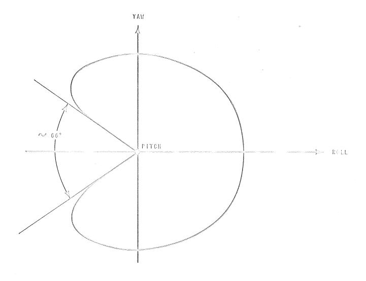
FIGURE 3 GENERAL CM ANTENNA RADIATION PATTERN
