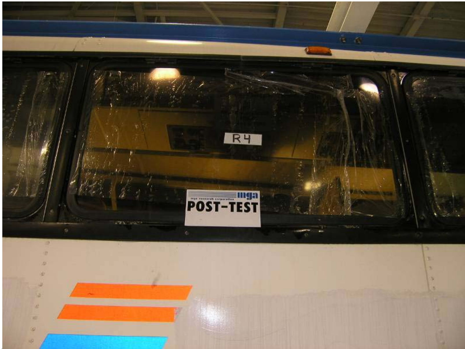
Post-Test Right Side Window 4 Exterior View
