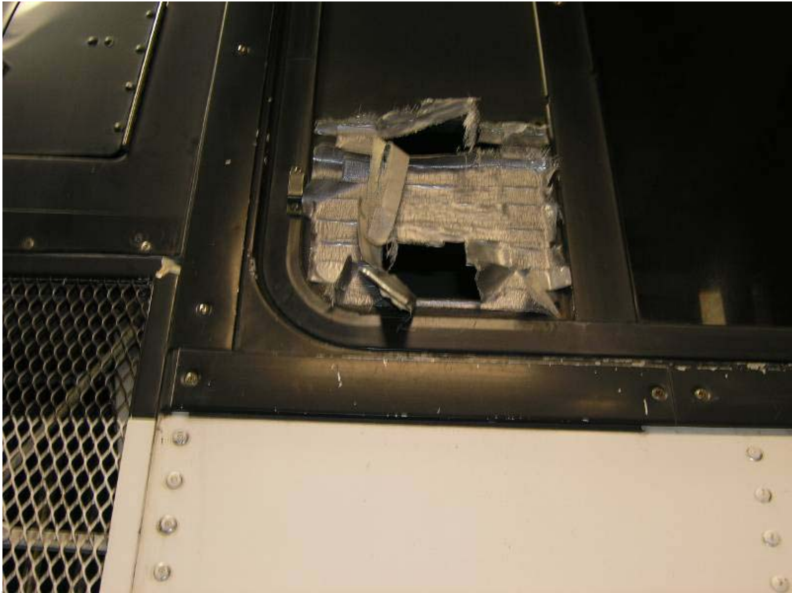
Pre-Test Close up View of Right Side Window 7 Damage
