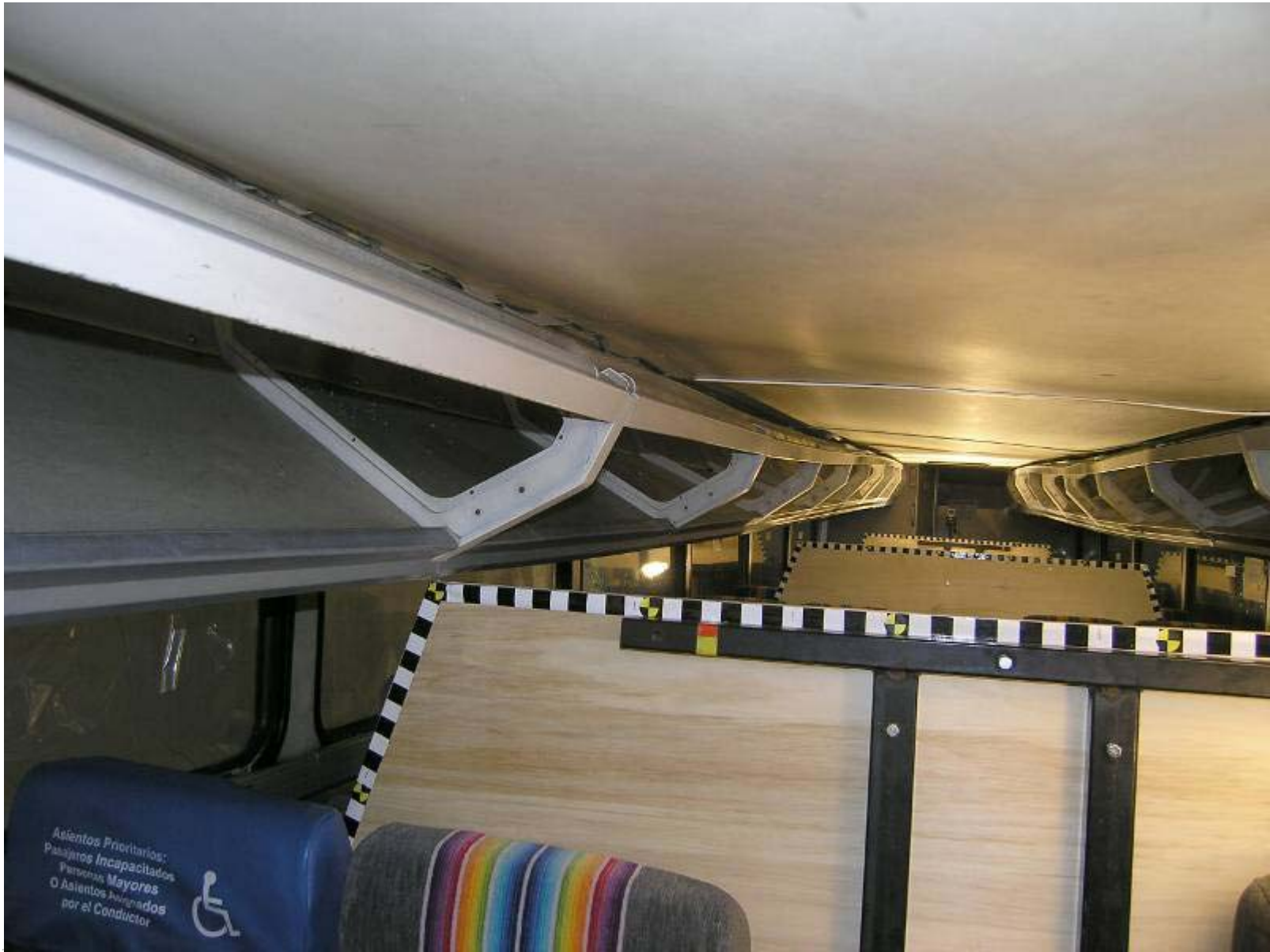
Post-Test Rear View of Bus Roof (Interior)
