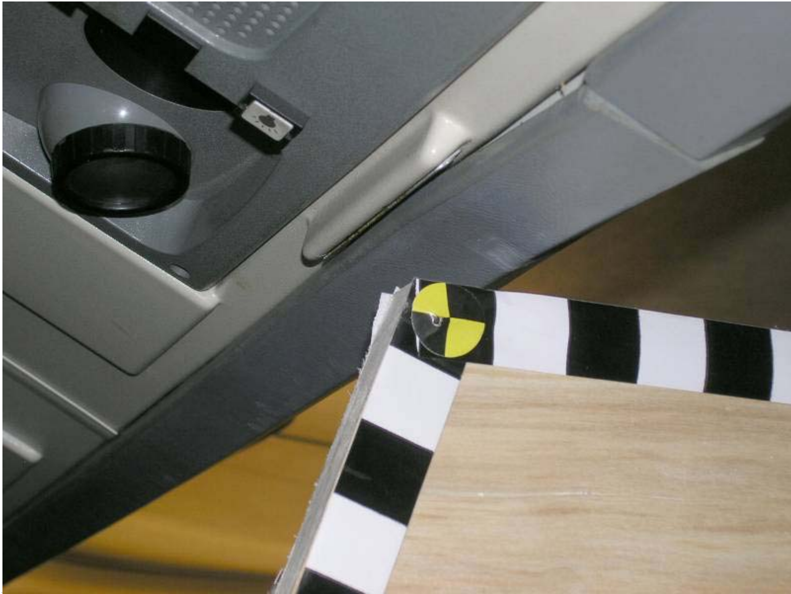
Post-Test Front Template Clearance View 1
