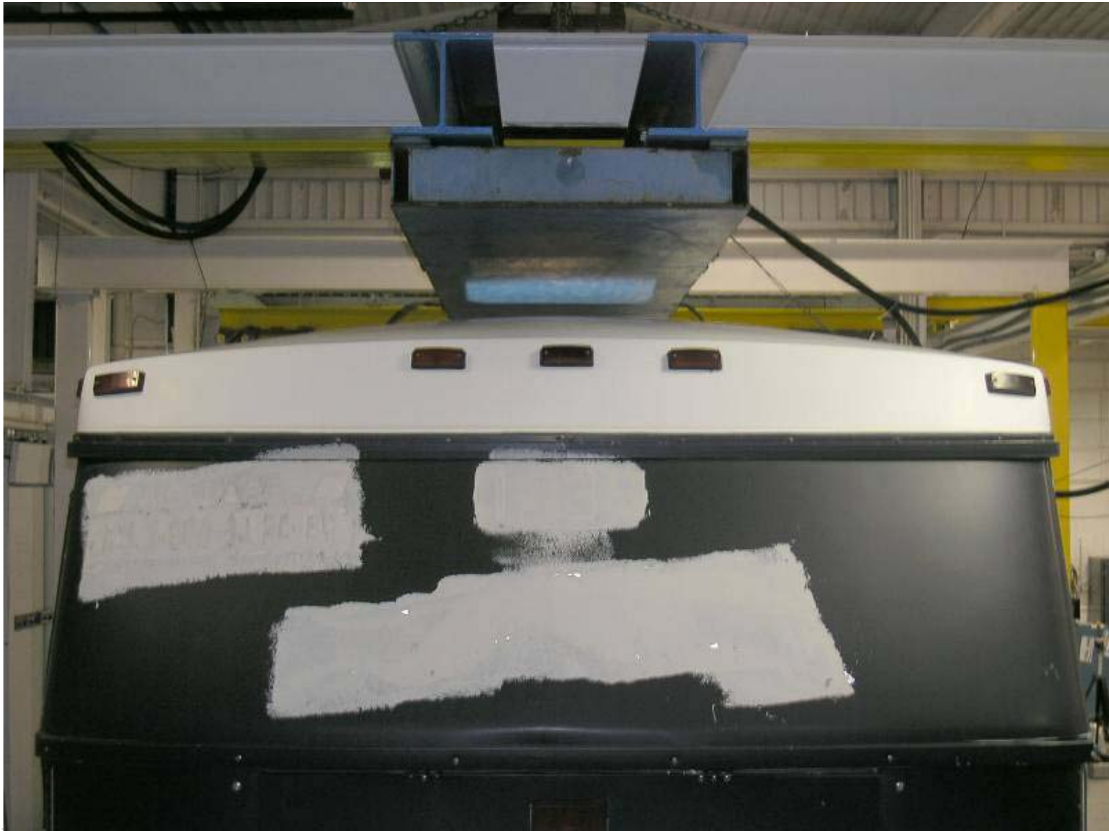
Post-Test Rear View of Bus Roof Close Up (Exterior)
