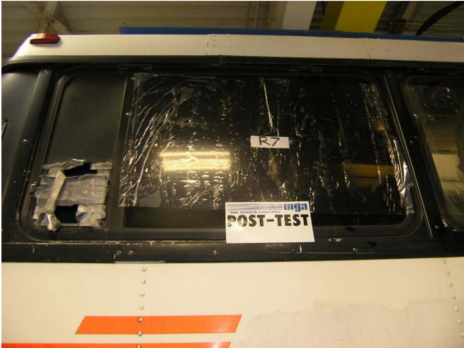
Post-Test Right Side Window 7 Exterior View
