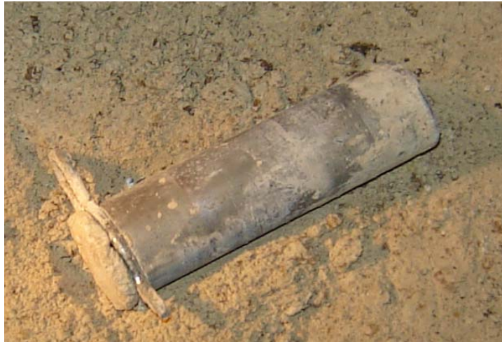
CLEVIS PIN THAT CAME OUT OF STEERING CYLINDER, ONE HAIRPIN STILL ATTACHED
