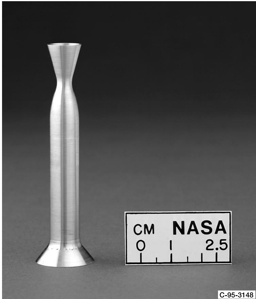
Figure 2.—Finished iridium liner.
