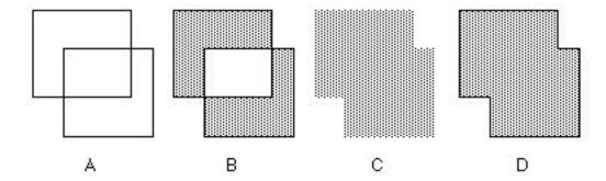
Figure A above shows two overlapping polygons. When the union of these two polygons is computed, we would like to get the polygon in figure D. In most cases, it is not difficult to compute results as in figure D. However, in the case of very convoluded polygons, and especially polygons that have one or more sides in common, computing the "right" answer as in figure D is quite difficult.
