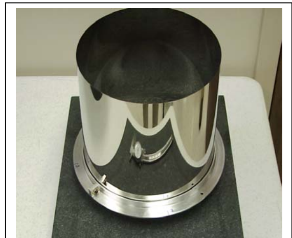
Figure 10: 100- \mu\text{m} -thick shell for multilayer stress tests
