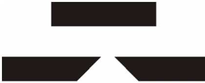
CADMIUM-FREE DESIGN OF THE TRIPLE-BOUNCE CHANNEL-CUT CRYSTAL WITHOUT THE “CAMEL CAVE” (ILL)
