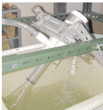
Flinabe would be used in beam-tube vortex flows, currently being studied in water-hydraulics experiments at U.C. Berkeley, shown in side and end views.
