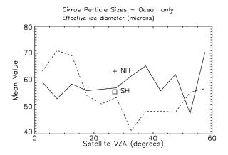
**Figure 4.** Mean CERES cirrus cloud particle size retrievals derived from northern hemispheric (NH, solid line) and southern hemispheric (SH, dashed line) MODIS observations as a function of satellite viewing zenith angle. The definition of cirrus is presented in the text. The plus sign and square represent the monthly means of all cirrus retrieved with a SVZA less than or equal to 60 degrees.
