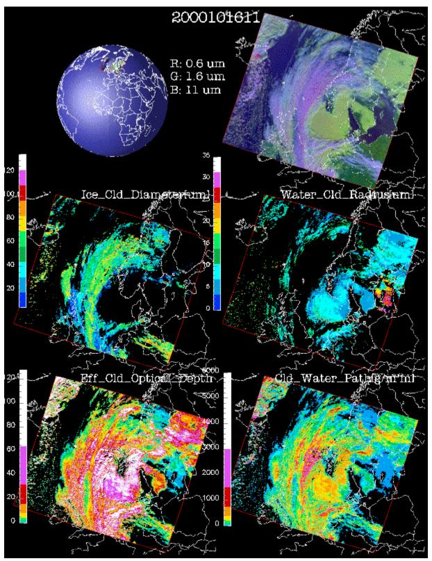
Figure 1. CERES cloud property retrieval from MODIS imagery on 16 October 2000. Top right hand figure is 3-channel composite highlighting the water cloud (green) and ice cloud (blue) regions. The images in the second row show ice particle diameter and water droplet radius in microns, while the bottom figure present the effective cloud optical depth and cloud water path.
