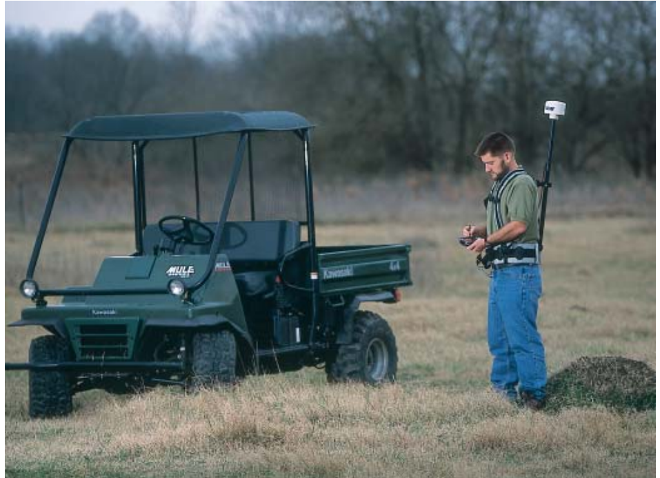
Technician John Davis uses a GPS unit to record the exact position of a fire ant mound. Mound position data are overlaid onto aerial digital images of the study site to determine mound visibility. Knowing the exact location of a mound also allows researchers to place parasitized ants back into their original colonies.
