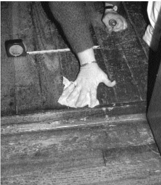
A dust wipe test can identify the active presence of lead. A moist towelette is used to collect dust and then is analyzed in the laboratory. If a property is freshly painted and well maintained and floors have been thoroughly washed and wet vacuumed, a dust wipe test can verify that it is lead-safe.
