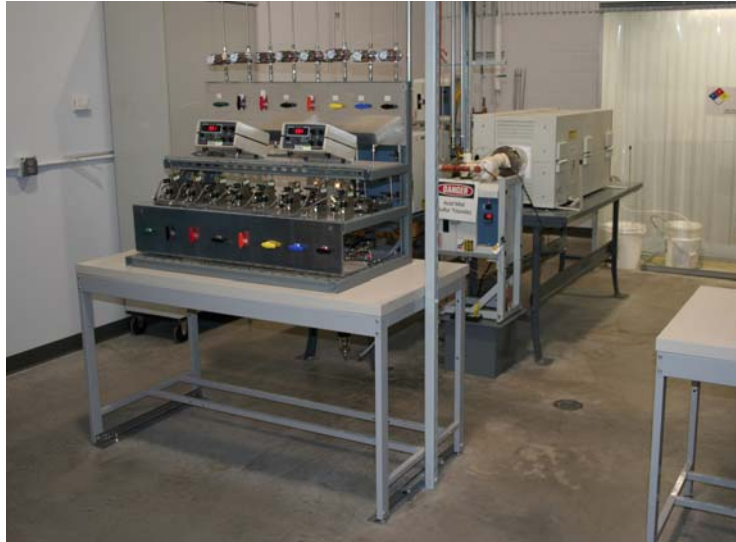
Figure 1 – Two Fireside Corrosion Testing Facilities Dedicated to the Current Materials Project.
