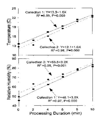
Fig. 1. Changes in temperature and relative humidity inside a debearder while processing Wyoming big sagebrush seeds (Booth et al. 1997).
