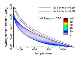
Figure 4: Joint probability density of temperature and fuel mole fraction in the flame cell for the domain of width 3.5 cm. Superimposed on the distribution is the temperature-fuel curve for two adiabatic, flat flames. Density is depicted in terms of percentiles of the distribution.
