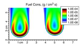
Figure 6: Fuel consumption in a pair of adjacent flame cells that persist for 4.5 s in the domain of width 7.5 cm.
