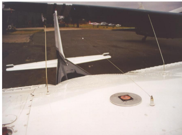
Figure 3 - SWIS Patch Antenna Mounted to Cessna 172 .
