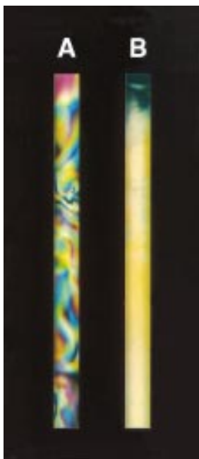
FIG. 8. Alignment of Rev filaments for fiber X-ray diffraction. (A) Rev filaments with an aspect ratio of about 18 and at a concentration of 150 \text{ mg ml}^{-1} in HSSE as initially drawn into a 0.2-mm-i.d. capillary. (B) Columnar phase obtained by shear alignment of A. The meniscus and some unaligned material are visible at the top. Capillaries were photographed between crossed polarizers at an angle of 45^\circ .
