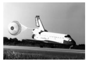
The orbiter Columbia returns to Kennedy's Shuttle Landing Facility, completing Mission STS-62 on March 18, 1994. All four orbiters in the Shuttle fleet are now equipped with a drag chute that is deployed during landing to assist in stopping and to provide greater stability in the event of a flat tire or steering problem.
