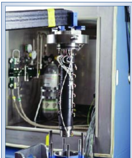
Figure 3: Instrumented Sample Sleeve Held Above the Cell Body
