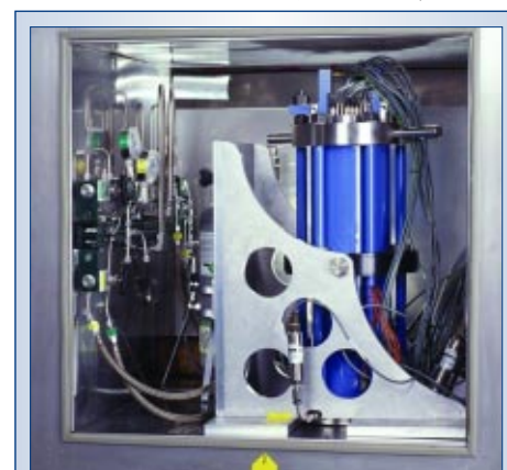
Figure 4: Assembled Reaction Cell Placed Inside Temperature-Controlled Chamber
