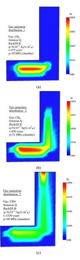
Figure 9. The advance of the free gas front in the emplacement chamber and in the gallery, three time steps.
