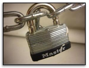
The shackle of this breakaway padlock is an example of a *frangible* element.
