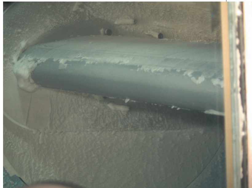
The NASA-developed Electro Expulsive Separation System (EESS) is shown in a testing chamber where it proved it could rid aircraft of ice layers ranging from thin frosts to thick glazes.
