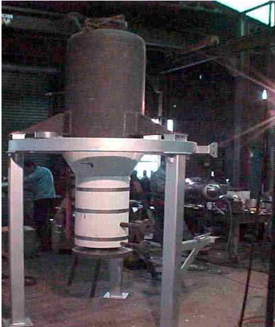
Figure 15. Fluidized-bed catalytic reactor
