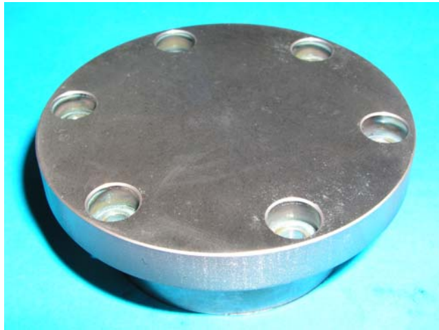
Figure 6 Surface view of the flat low fixed CuCrZr mirror , which was initially polished at \lambda , after plasma exposure
