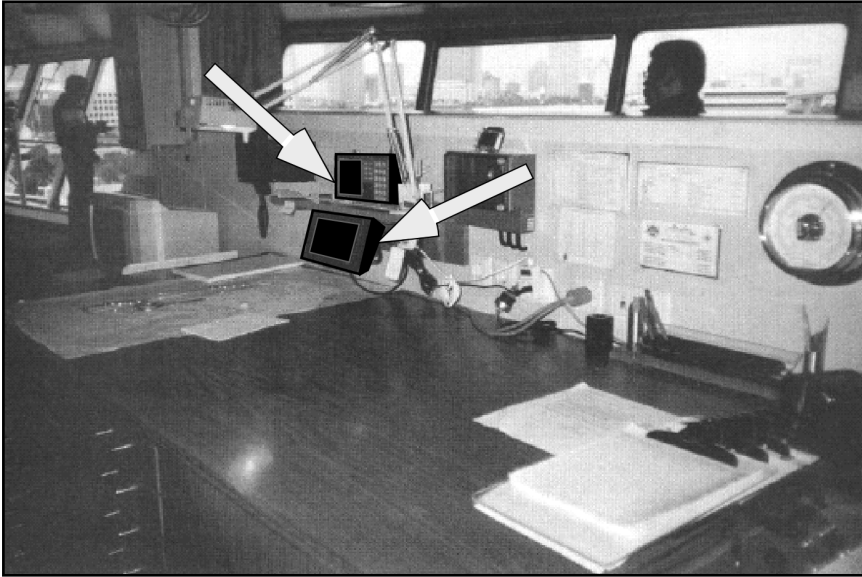
Figure 8.2. The chart table and the bridge. The left arrow points to the GPS unit, the right arrow points to the LORAN-C unit. Source: National Transportation Safety Board (the photo has been enhanced).
