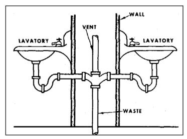
Figure 9.11. Back-to-back Venting [Sink]
