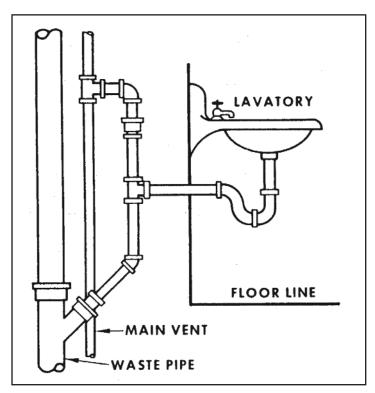
Figure 9.12. Wall-hung Fixtures
