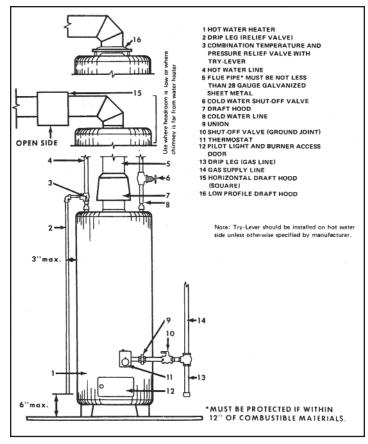
Figure 9.3. Gas Water Heater [1]
