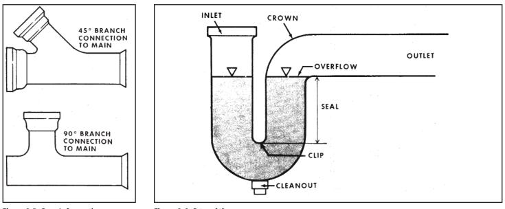
Figure 9.5. Branch Connections
