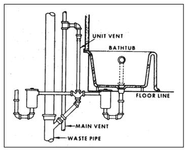
Figure 9.13. Unit Vent Used in Bathtub Installation
