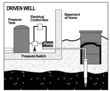
Figure 8.2. Cross Section of a Driven Well
