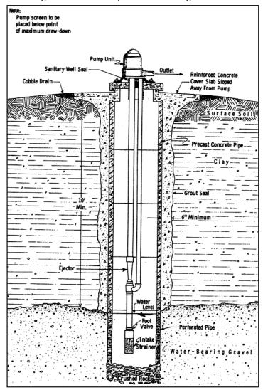
Figure 8.5. Recapped and Sealed Dug Well [1]
