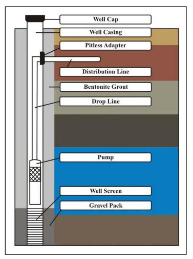
Figure 8.6. Drilled Well [4]
