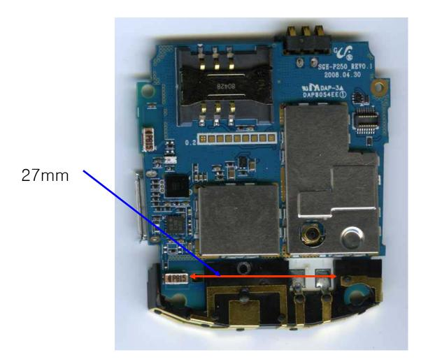
No difference of distance between bluetooth antenna and PCS1900 antenna for each case of slide up and down, because antennas are in the same plastic all together.
