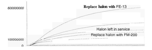
There is a slight advantage to removing Halon 1301 from service and replacing it with FM-200. The advantage arises largely from reductions in emissions caused by improvements in equipment, assuming that equipment (valves, seals, etc.) will improve when systems are replaced.
