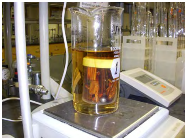
Figure 20- Overview of Pinus taeda chips penetration test with modified cooking liquor at 70°C.
