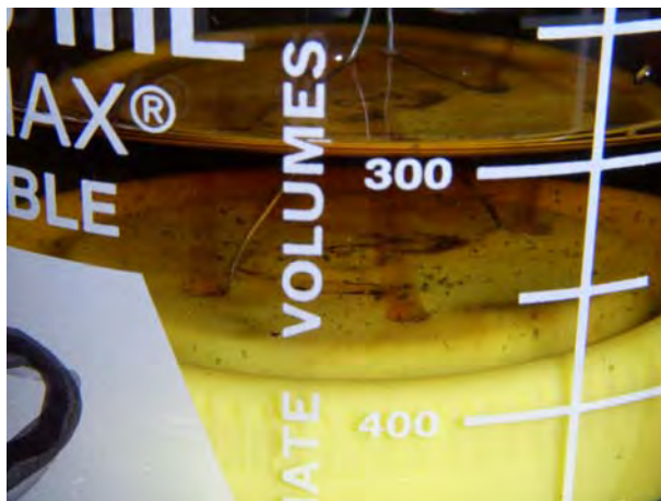
Figure 21- View of material going out from Pinus taeda basket chips after 60min. of treatment with modified cooking liquor at 70°C.
