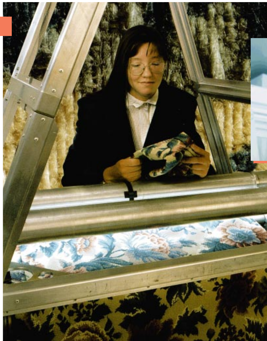
A camera (inset) is mounted at the top of this A-frame structure, which is part of the demonstration unit for computer-aided fabric evaluation. Behind the A-frame is a closeup of the fabric that summer student Jessica Bayliss is inspecting.
