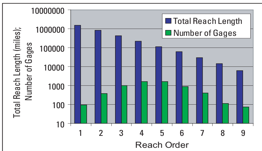
Figure 4. Estimated distribution of total stream-reach length (Leopold, 1962) and number of streamgages (in 1996) across reach orders for the 48 conterminous States. (Reach order associated with each streamgage was estimated on the basis of drainage area. First-order reaches average 1 square mile in area, and drainage area increases by a factor of five with each increase in stream order.)
