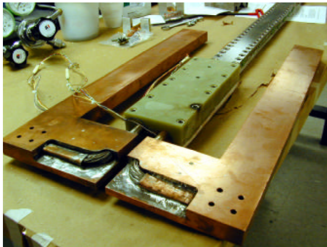
Fig. 8. Cable critical current sample holder before insertion into test station.
