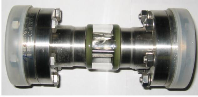
**Figure 1.** Packaging of the lithium lens inside a hermetic enclosure.
