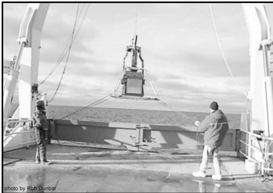
Herb Baker, left, and Patrick Whaling deploy a box coring device off the back side of the Nathaniel B. Palmer during the ROAVERRS cruise.
