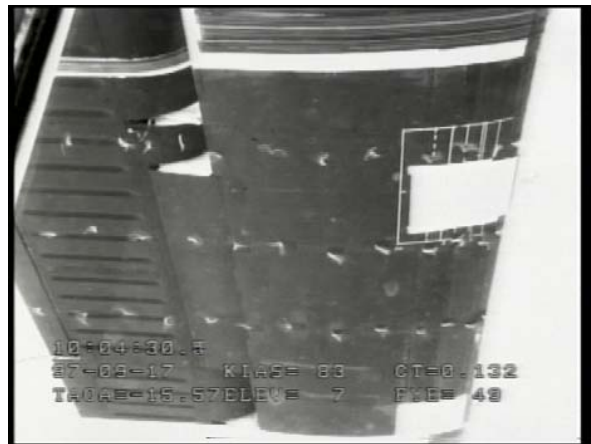
Figure 2. Top: Technician applying artificial ice shape to the leading edge of the tailplane. Bottom: Flow reversal as the ice-contaminated tail becomes fully stalled.
