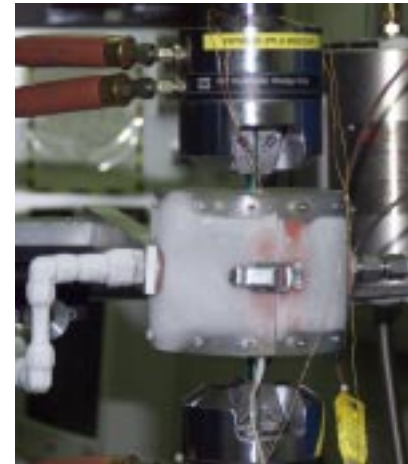
Cold Test Chamber ( T = -40^{\circ}\text{C} )
