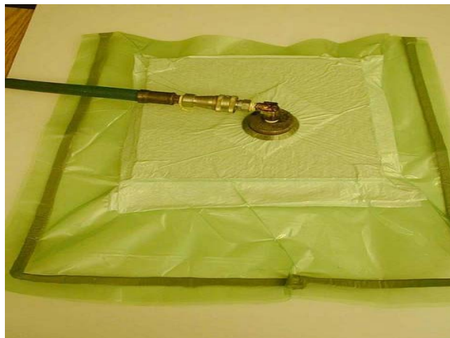
FIGURE 3. VACUUM BAGGING ADHESIVE TEST PANELS
