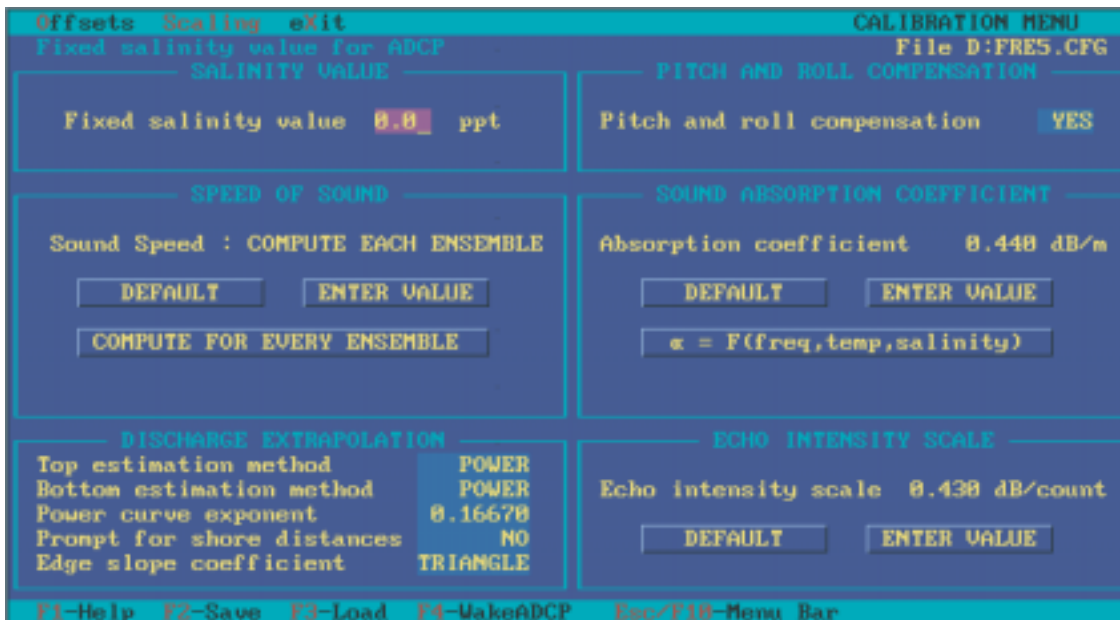
Figure 5.6. Calibration scaling submenu screen. ADCP, acoustic Doppler current profiler.
