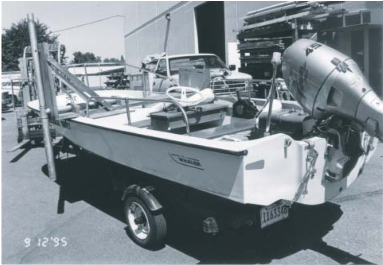
Figure 4.10. Side-swing mount on a 4.5-meter (15-foot) Boston Whaler for an acoustic Doppler current profiler.
