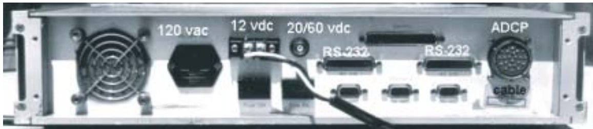
Figure 4.4. Front and rear view of an R.D. Instruments, Inc., acoustic Doppler current profiler deck unit.
