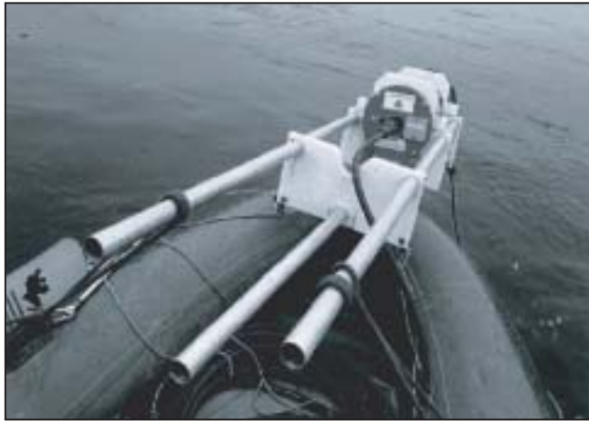
Figure 4.11. Acoustic Doppler current profiler mount for an inflatable dinghy.
