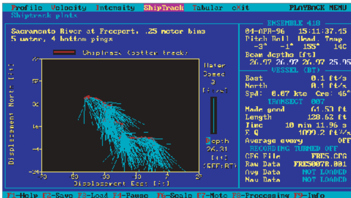
Figure 8.2. Transect software shiptrack plot of an anchored vessel.
