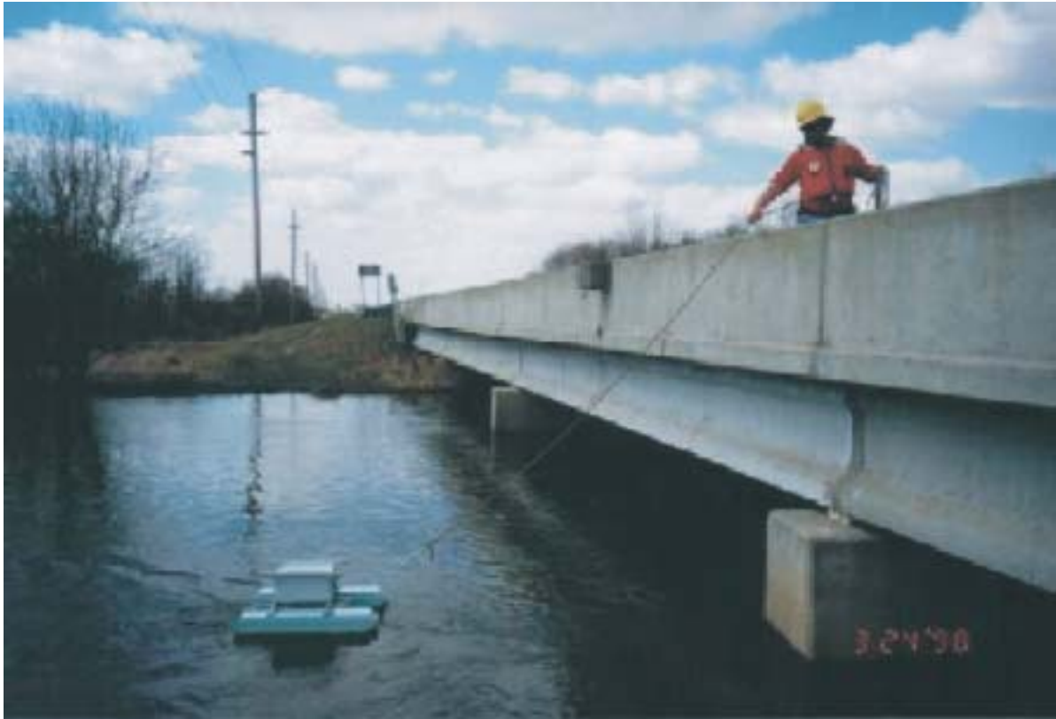
Figure 4.6. Tethered acoustic Doppler current profiler discharge measurement platform.
