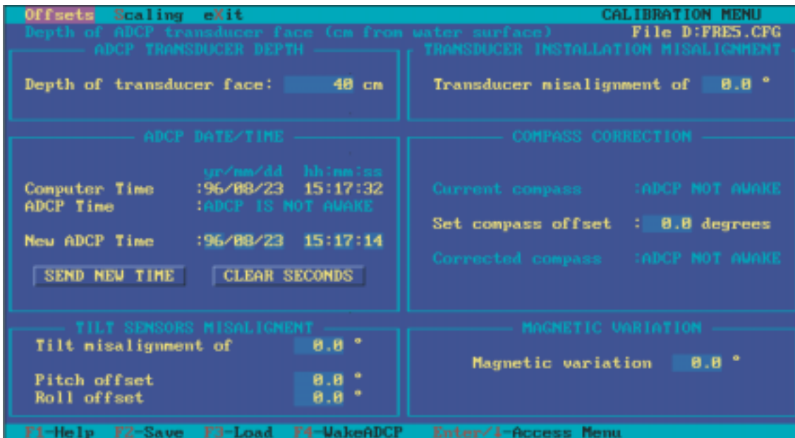
Figure 5.5. Calibration offsets submenu screen. ADCP, acoustic Doppler current profiler
