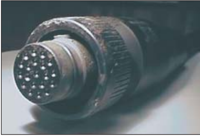
Figure 4.5. Connector cable for attachment of R.D. Instruments, Inc., broad-band acoustic Doppler current profiler to accompanying deck unit.
