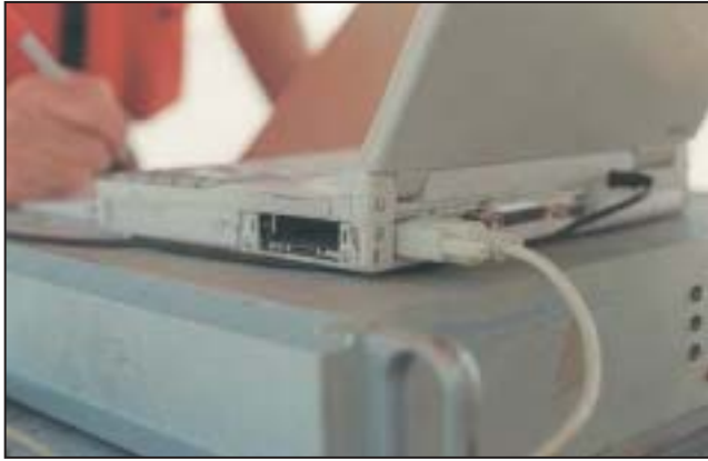
Figure 4.13. Laptop computer with missing plastic doors and port covers.
