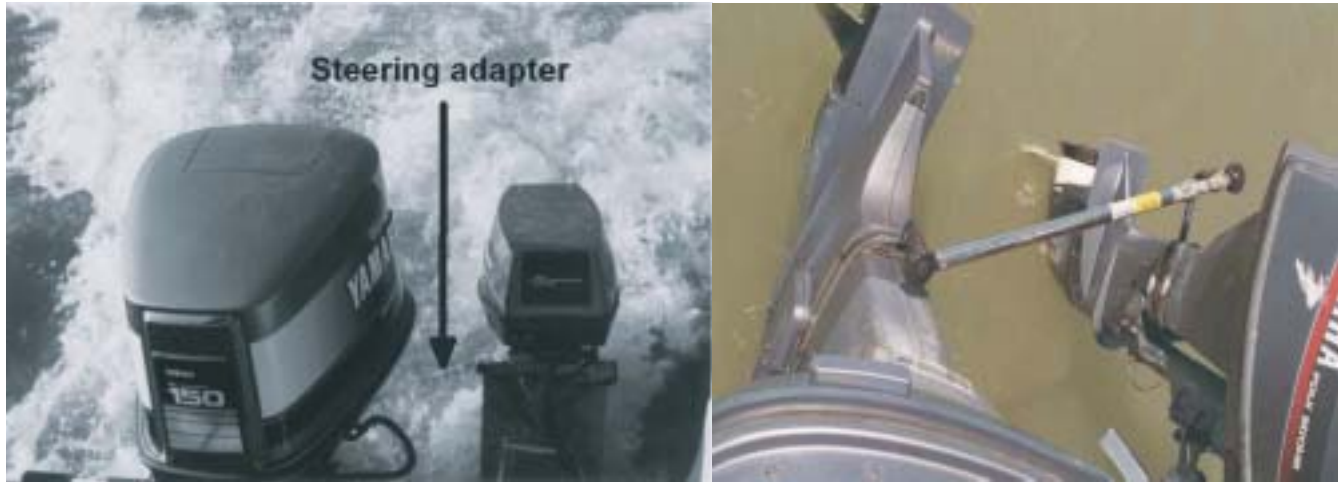
Figure 4.24. Two views of a steering adaptor that connects the trolling motor to the main engine.
