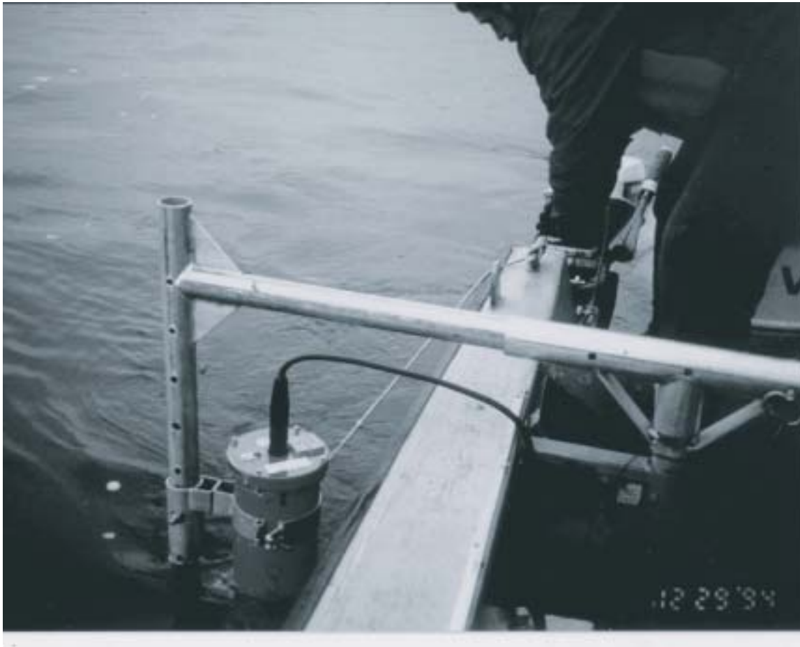
Figure 4.20. Swing mount variation used by the U.S. Geological Survey Illinois District.
